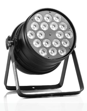
A high power LED Par in Aluminium housing with 18x12 W RGBWA+UV (6-in-1) LEDs. Equipped with DMX in/out for daisy chaining multiple units together. It has preset programs that can be used in stand-alone mode. In the DMX settings there is the choice of a few channel modes with preset colours. The Aluminium housing and double stand make the fixture ideal for rental features, being lightweight and easy to setup.
